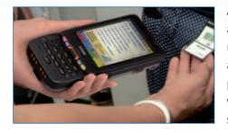
As the first industrial PDA with the operation system Windows Mobile 6.5 and 3.5G Wireless WAN, WLAN and Bluetooth the IT-800 can be used extremely flexible. Along with the rapid data communication the terminal offers also telephone functionality and can therefore replace mobile phones completely. Further features are GPS for locating the exact position, a camera with autofocus and flash for fast image documentation as well as a laser scanner or CMOS imager for 1D or 2D codes.
