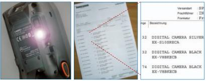
camera with autofocus and flash. The pictures can be submitted immediately to the head office using the integrated WWAN module. If necessary GPS location information, daytime and date can be added to the pictures.
